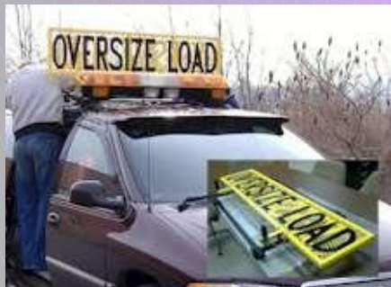
THE OVERSIZE LOAD SIGN EASILY FOLDS DOWN WHEN NOT NEEDED AND IS PINNED IN PLACE.
